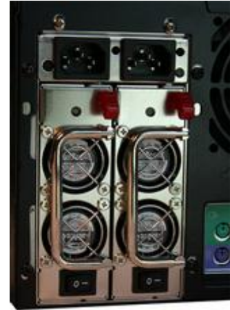
OPTIONAL REDUNDANT POWER SUPPLY
